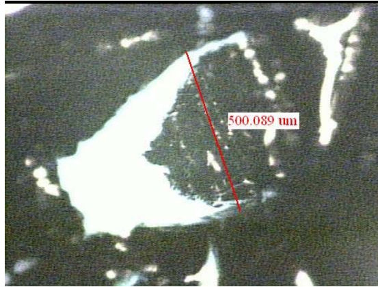
Fig. 44. The delamination on the solid surface.
